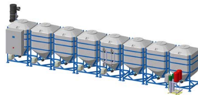
AquaCycle 12500 Recycling capacity 10000 Liters/Day AquaCycle_04.tif
